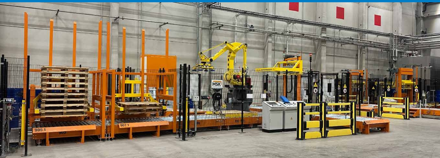
Palletising system for placing empty drums on pallets and strapping them.
