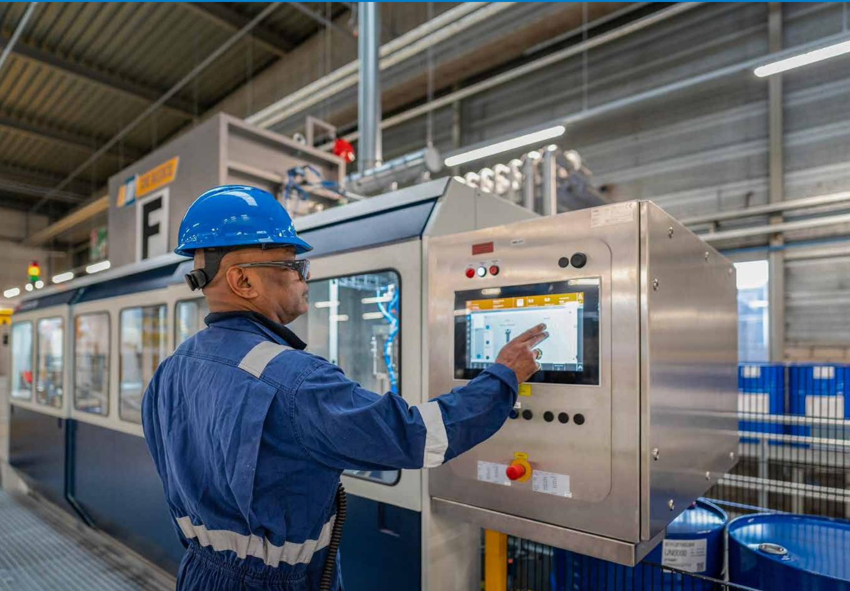
Feige T86 filling machine for drums, with 6 filling stations.
