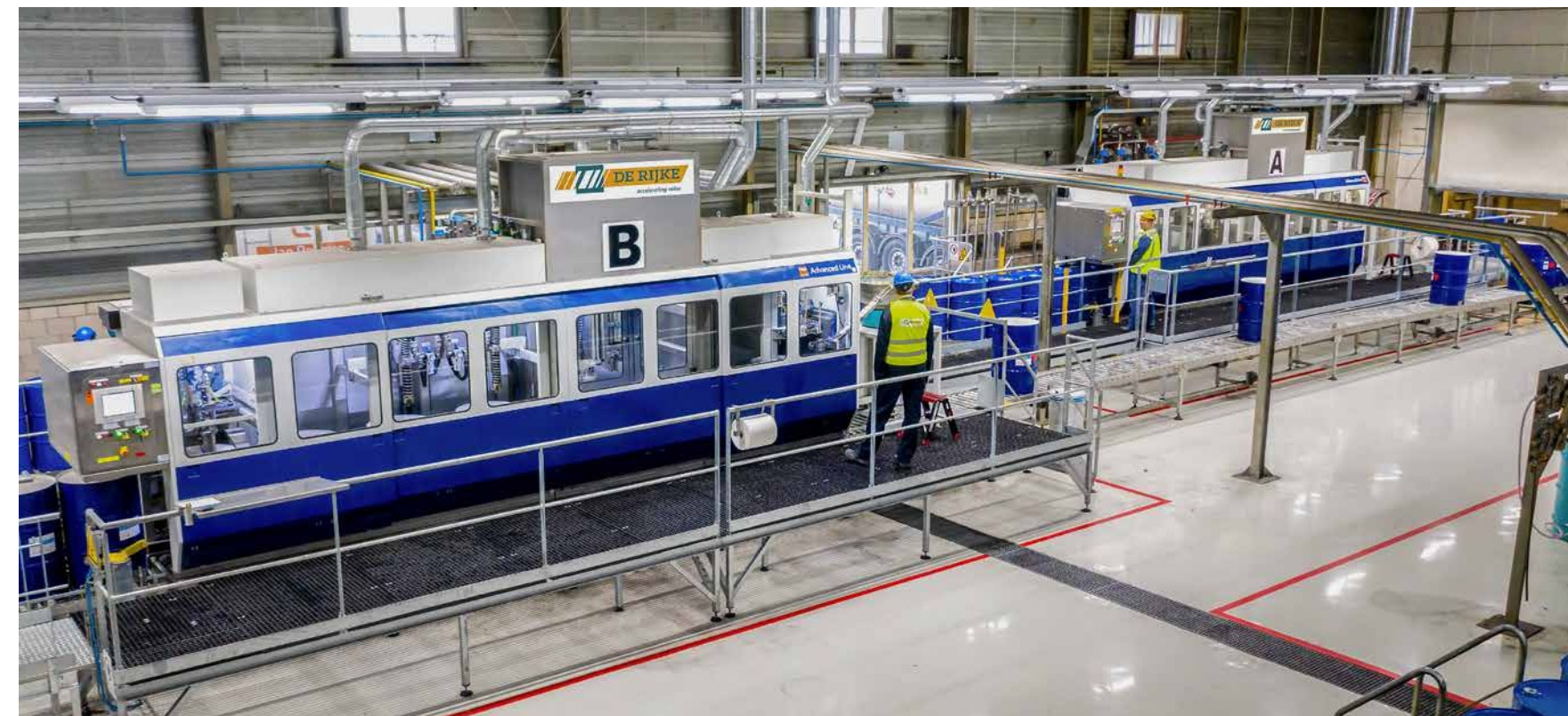
Feige's T88 filling machine can fill 125 barrels per hour.
